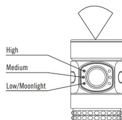
If the brightness level indicator fluctuates, it means that the current brightness level is at least 45% or higher.
