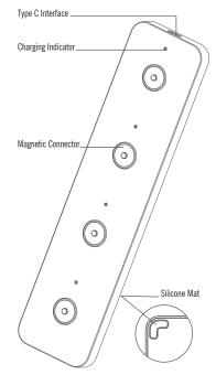
After connecting the Omino to the readily plugged power adapter with a USB cable, you can charge the compatible devices at any charging port of the Omino.
