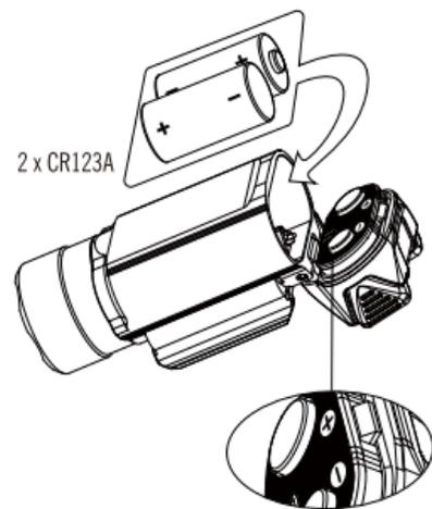
3. Hold the tailcap firmly and then close the spring lock.
