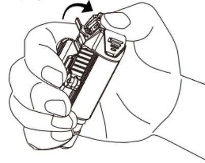
Before first use, please open the tailcap as the picture shown, take off the insulating film then cover the tailcap.
