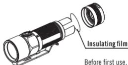
Before first use, unscrew the tailcap and take off the insulating film.
