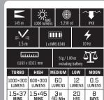
All above specifications are test results based on ANSI/NEMA FL1-2009 Standard. The tests are performed using the battery included in the flashlight.
